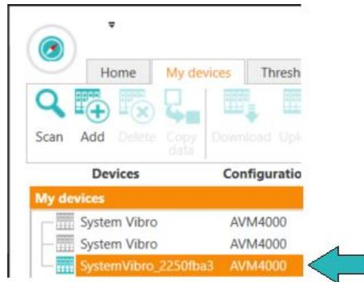
13. Double-click on the name of the found device, this will open the system configuration in the main application window
