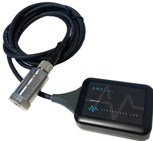
PC → USB/USB C cable → AVS USB CON adapter → sensor
