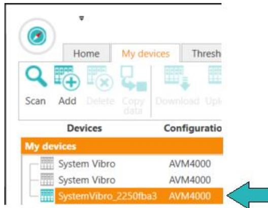
13. Double-click on the name of the found device, this will open the system configuration in the main window of the application
