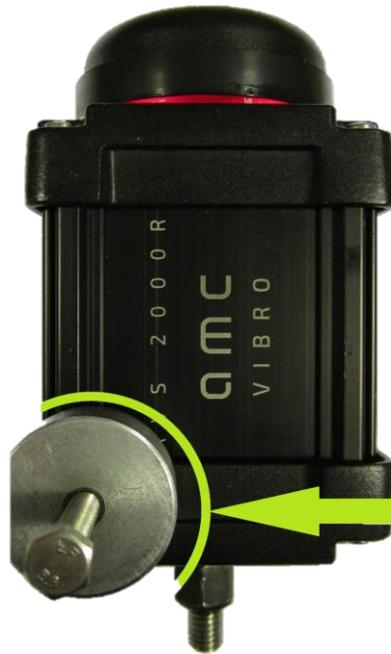
Figure 3. Wake up the vibration sensor
