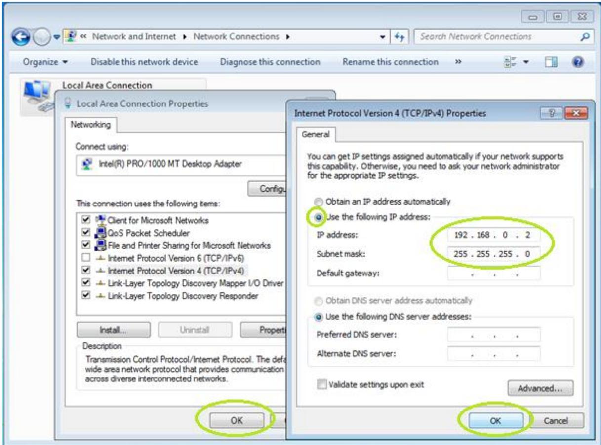
Figure 44. Computer IP address
