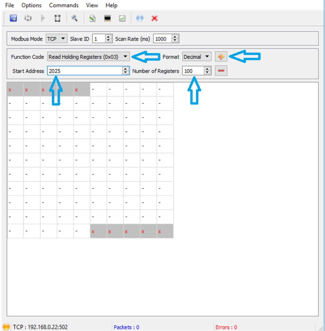
Figure 31. Function settings, start address, number of registers
