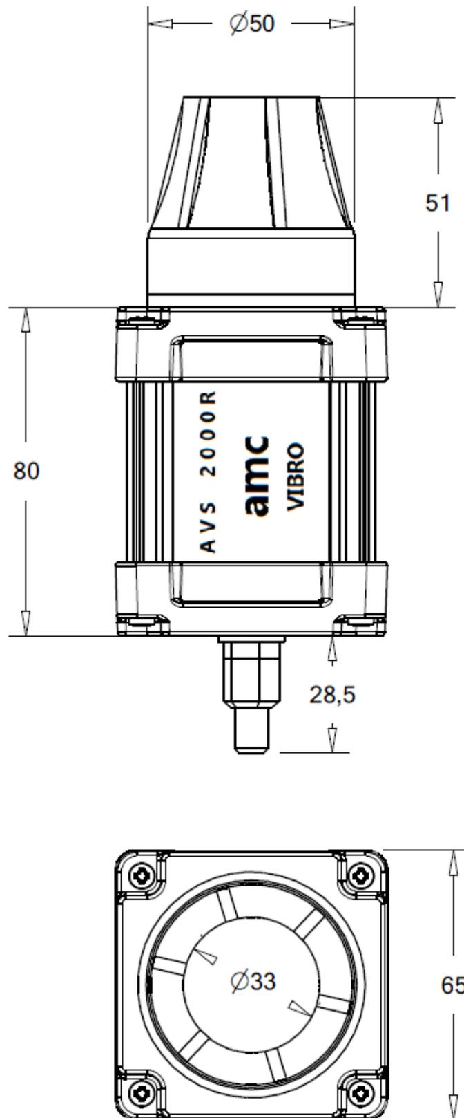
Figure 6. AVS 2000R dimensions in millimeters
