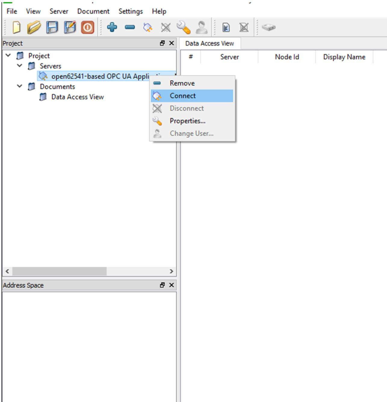
Figure 36. Connecting to new server
