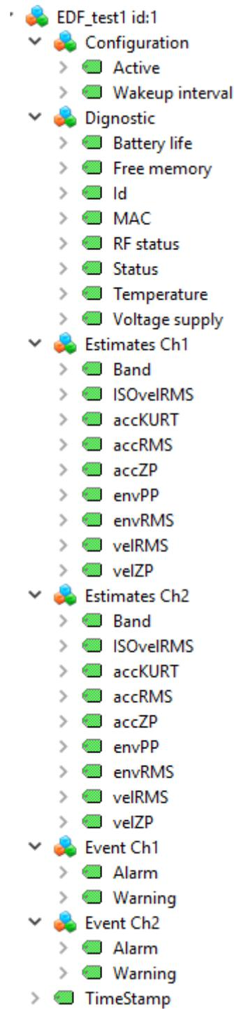
Figure 27. The OPC structure for the vibration sensor
