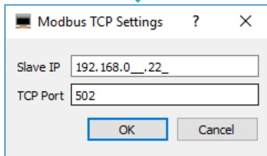
Figure 29. Defining IP and port for Modbus TCP
