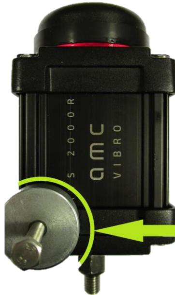
Figure 45. Wake up the Vibration sensor
