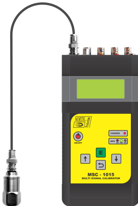
Figure 125 Testing IEPE Sensor
