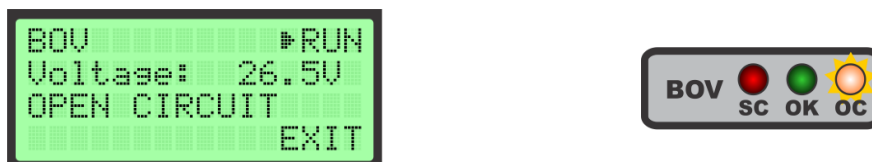
Figure 61 BOV Test - OPEN CIRCUIT
