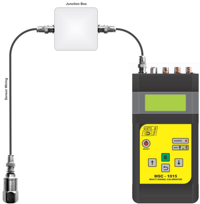
Figure 126 Testing IEPE Sensor including Cables and Junction Box
