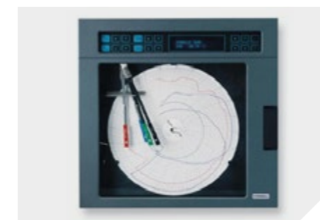
Analog chart recorders were used for trending and could be circular, such as shown here, or linear on roll of paper in so called “strip chart” format. Image courtesy of Eurotherm Chessell.
