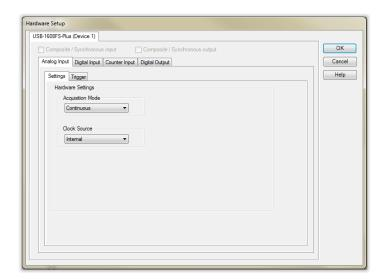
The only relevant tab here is *Analog Input*. After clicking the following tabs will be displayed: *Settings* and *Trigger*.
