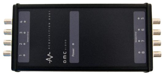
Inputs – BNC inputs used to connect IEPE standard sensors
