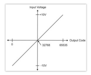
The offset error is measured in the mid-point of the measurement range. In an ideal case, an input signal of 0V should cause the converter to return the value of 32768. Any other result means an offset error. For the  $\pm$  10 V range, the maximum offset is  $\pm$  1.66 mV.
