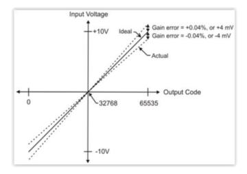
Adding the offset and the gain errors produces the device's total measurement error.
