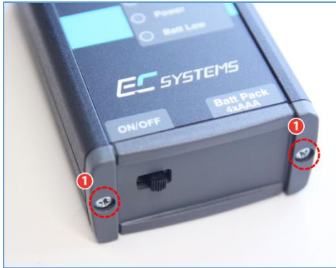
Figure 4.1 View of the screws allowing access to the battery compartment.
