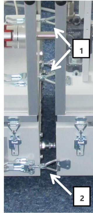
Figure 5.13 // Horizontal and vertical clamps
