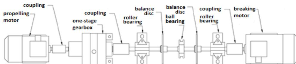
Figure 3.1 // The kinematic chain of the AV TEST BENCH 2
