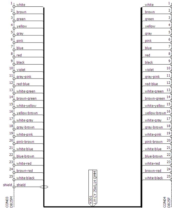
Figure 5.6 // Wiring diagram of a cable
