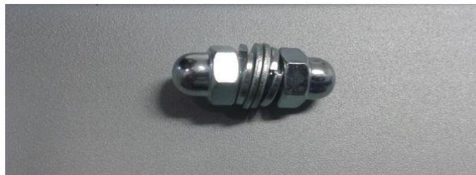
Figure 5.16 // Unbalance element
