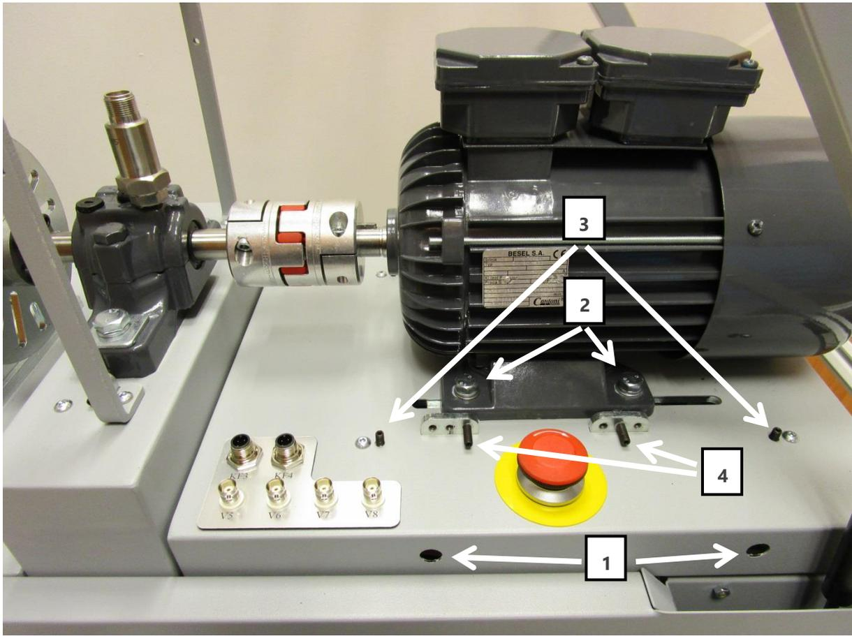
Figure 5.12 // Alignment of braking part
