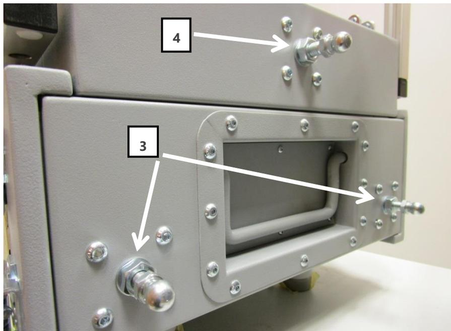
Figure 5.14 // Alignment of propelling part with braking part
