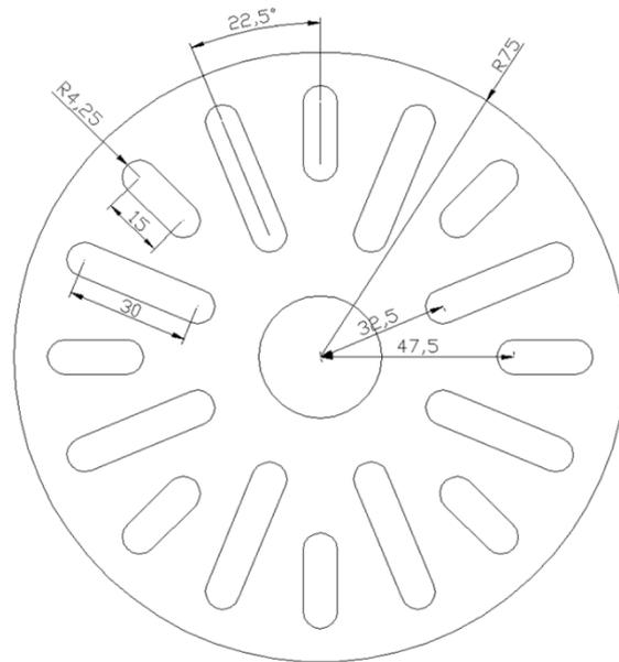
Figure 5.17 // Dimensions of unbalance disc
