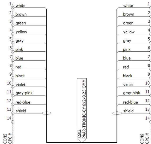
Figure 5.9 // Wiring diagram of a cable
