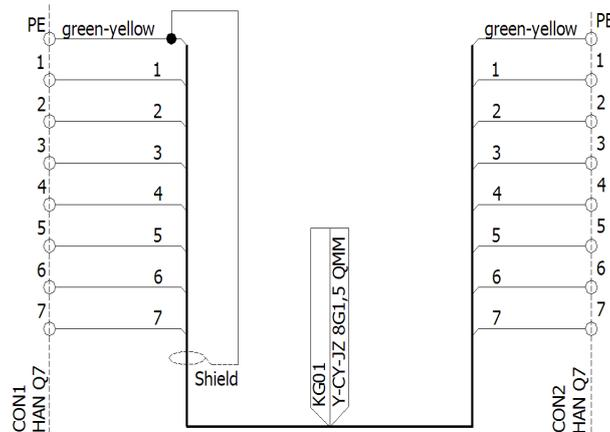
Figure 5.3 // Wiring diagram of a cable
