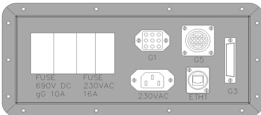
Figure 3.8 // The rear panel of the propelling part (panel B)
