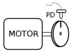
The shaft rotation is divided into 36 sections every 10<sup>o</sup> that the vibration acceleration (0-Peak and RMS) and the vibration velocity values (0-Peak and RMS) are calculated in. Furthermore, the device provides minimum and maximum value that occur within all sections. Estimates based on sections of full rotation can also be sources of warnings and alarms.
